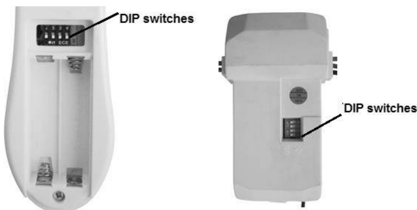
Fig. 9 Remote battery compartment
